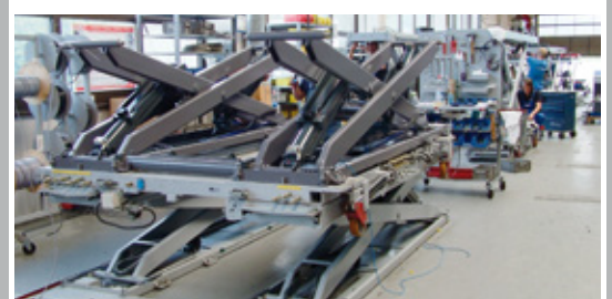
State-of-the-art production lines as an example: Scissors lifts production line
