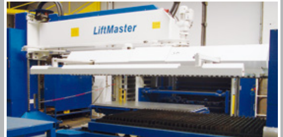
Automatic raw material pick-and-place system for precision laser cutting
