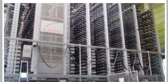
Electronically controlled high-bay warehouse
